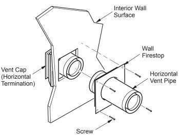
Figure 12 - Connecting Vent Cap with Horizontal Vent Pipe
